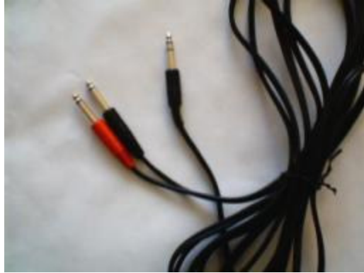
Picture 1. A standard stereo 1/4" jack cable split in two 1/4" mono jacks, also known as INSERT CABLE .
